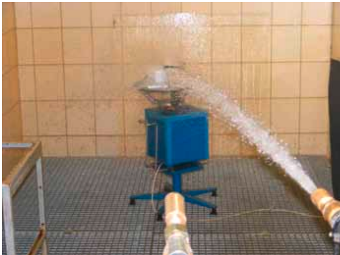
Figure 9 Loading by water IP X6, exemplarily
